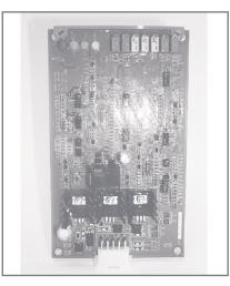
Compact, highly responsive driver boards for long life operation of PML valve driver joysticks. Smooth centering, EMC protection and a host of safety features built-in.
